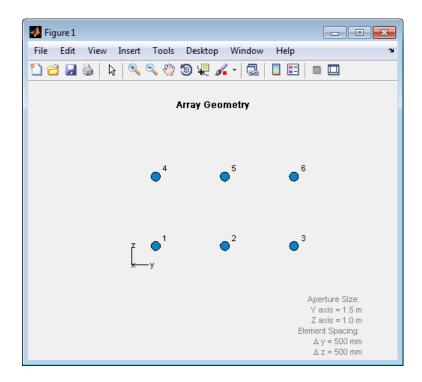
Create and view an array consisting of three 2-element linear subarrays parallel to the *z*-axis. Use the numbers in the plot to help form the matrix for the SubarraySelection property. Also, find the phase centers of the three subarrays.
