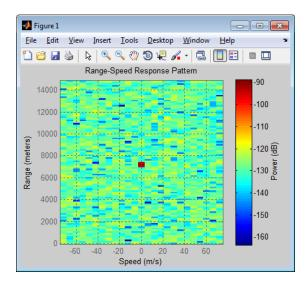
The plot shows the stationary target at a range of approximately 7000 m.
