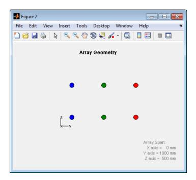
Create and view another array consisting of two 3-element linear subarrays parallel to the *y*-axis. Find the phase centers of the two subarrays.
