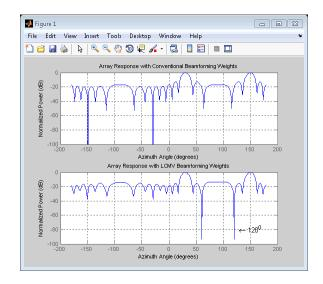
The LCMV beamforming weights place a null in the array response at the arrival angle of the interference signal.
