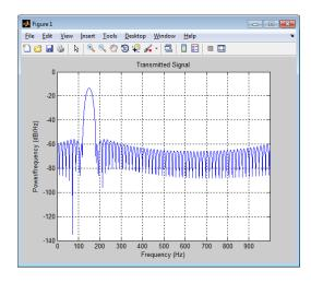
Plot the spectrum of the propagated signal. The peak at 250 Hz reflects the frequency of the signal plus the Doppler shift of 100 Hz.
